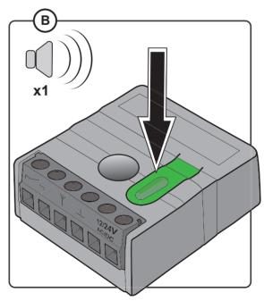
B. Within 10 seconds the button on on the pilot must be pressed. Hold until a sound signal is heard.
