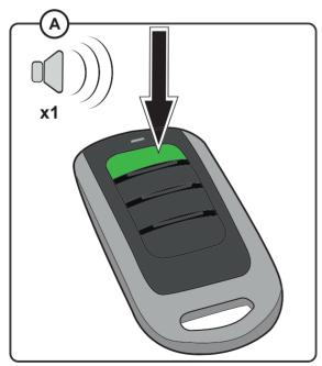
A. Press and hold one of the four buttons on the controller that shall interract with the pilot. Hold until a sound signal is heard.
